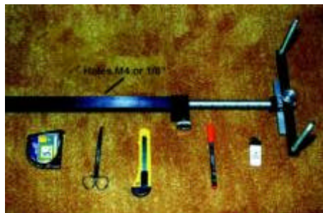
Fig. 1 The string jig. Note some simple tools you will need; measuring tape, scissors, X-acto knife, lighter, and marker.
